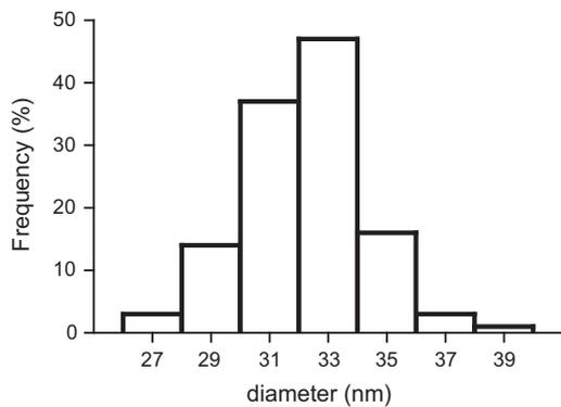
**Fig. 1.** The histogram shows CuONPs size distribution. The size for CuONPs ranged from 27 to 39 nm with an average particle size of 33 nm. Size distributions were obtained from 6 independent DLS measurements.
